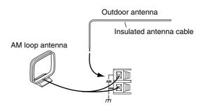
Outdoor AM antennas work best when installed outside horizontally, but good results can sometimes be obtained indoors by mounting the antenna horizontally above a window. Note that the AM loop antenna should be left connected.
